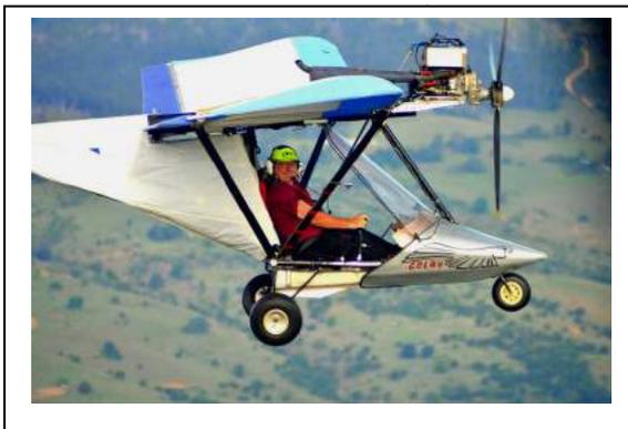
climbing turn I notice a very marked tendency to overbank, a function of the light wing loading. Level turns hold no surprises and 60° turns just seem to happen.
