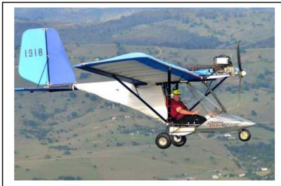
The test flight had been uneventful. Its take off proved as short as the book suggested and climb-out at V<sub>y</sub> was phenomenal. In cruise, I had to pull the RPM to 5300 to cruise level at 55 knots – playing with the throttle quickly demonstrated that if I applied full power I could exceed the V<sub>ne</sub> of 65 knots even in a climb. Visibility was superb; the low pod-nose profile gave fantastic view ahead. In fact, maintaining height and 55 knots
