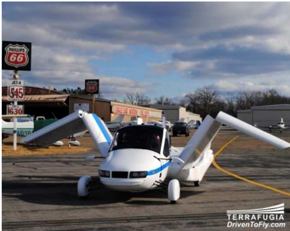
With its wings folded, the Terrafugia Transition can operate on the same roads as automobiles.
